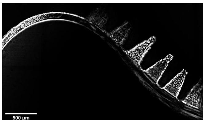
Figure 1. Epithelial cells (nuclei in grey) on PDMS pillars on a magnetic composite membrane curved by the application of an external magnetic field.
