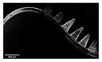
Figure 1. Epithelial cells (nuclei in grey) on PDMS pillars on a magnetic composite membrane curved by the application of an external magnetic field.
